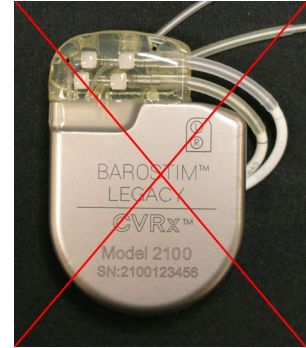
Incorrect placement of lead behind IPG
