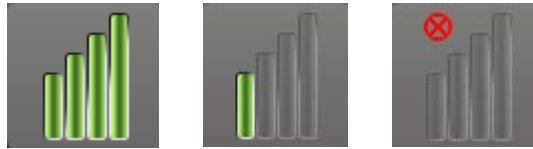
Figure 9: Link Quality Indicator (Excellent, Poor, No Link)
