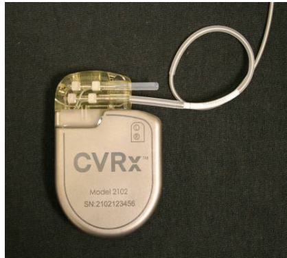
Figure 20: Correct Placement of Excess Lead Body
