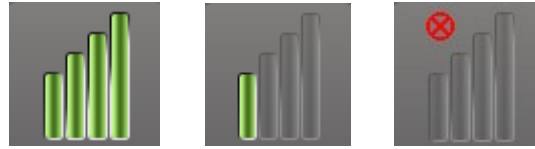
Figure 10: Link Quality Indicator (Excellent, Poor, No Link)
