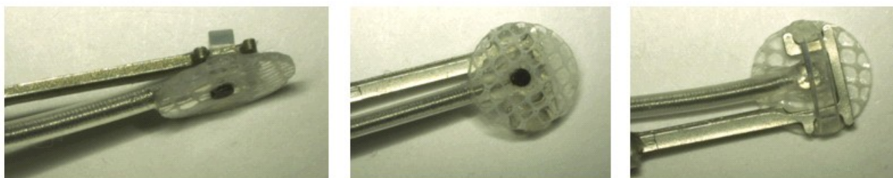
Figure 15: Buckle lead engaged in Buckle Implant Tool
